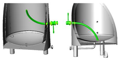
Special system is intended to pump beer from different levels in tank. With decantator user can use BBT as fermentation tank and storage tank. Users usually use BBT to maximize volumen per square meter.
