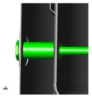
Special insertion of thermowell for holding temperature probe. With this special insertion there is no welds of thermowell and also there are no threads.
