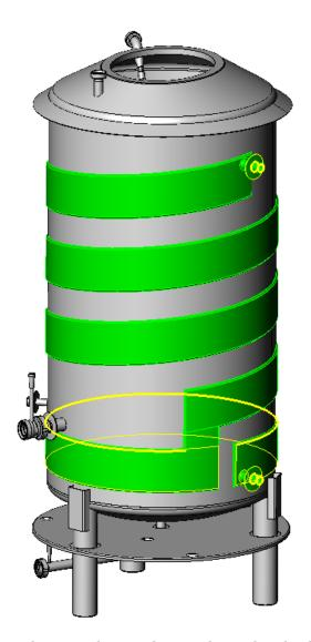
Cooling liquid is forced to circulate and to go through cylindrical part and on low point on wall is special cooing stripe to increase cooling efficiency on this low part of tank. High tech production of BBT enables better cooling performance.
