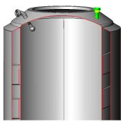
DN25 connection for air lock, safety valve and pressure release valve.
