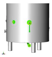
$2x\ DN25$  connection for butterfly valve and DN15 connection for sampling tap.
